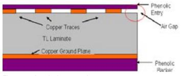
Figure 5 - A typical rout stack
