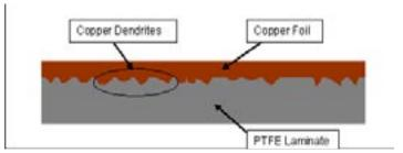
Figure 1 - Illustration of copper laminated to PTFE surface
