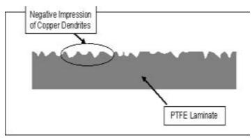
Figure 3 - Illustration of PTFE surface remaining after copper removal / etching
