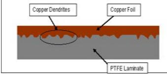
Figure 2 - Illustration of copper laminated to PTFE surface
